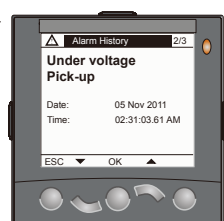
Alarm pick-up and drop-out.
